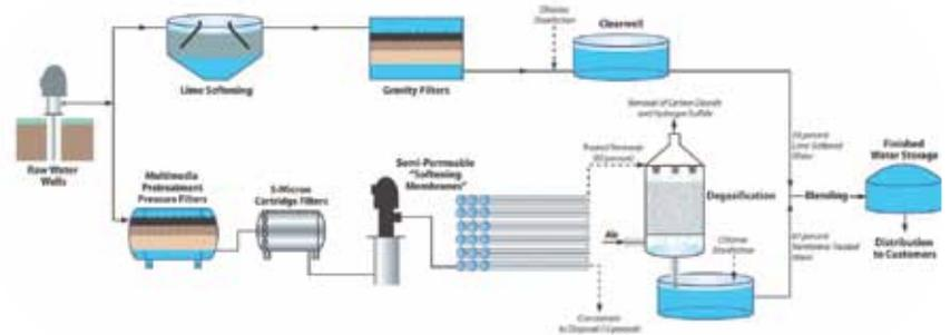
removed using a degasifying technology. The membrane softened water is also disinfected with a chlorine compound and blended with the lime softened water. The combined processes produce high quality water that is pumped through the distribution system to our customers.
